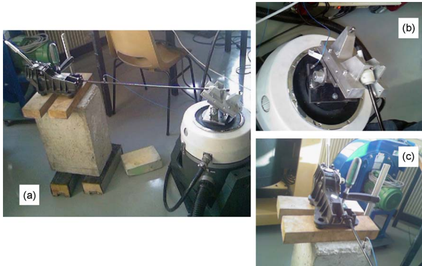
Fig. 6. Experimental setup used to test the outer housing: (a) complete setup, (b) attachment on shaker and (c) attachment on shift box.
