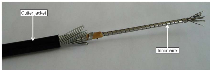
Fig. 2. Close up of the cable structure.
